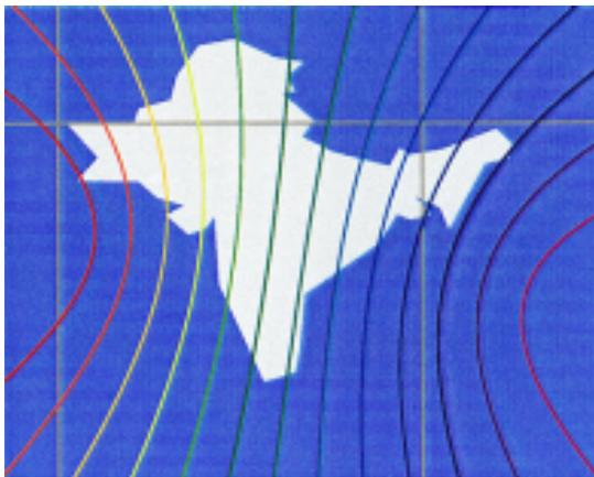
Figure 3. Contours, spaced at 2 ms intervals, of relative delay between single-hop skywave transmissions from Oman (MF) and Thailand (HF).
