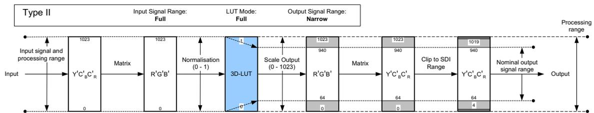
**Figure 2 - Type II signal-scaling, intended for full-range input signals (e.g. some PQ variants)**
