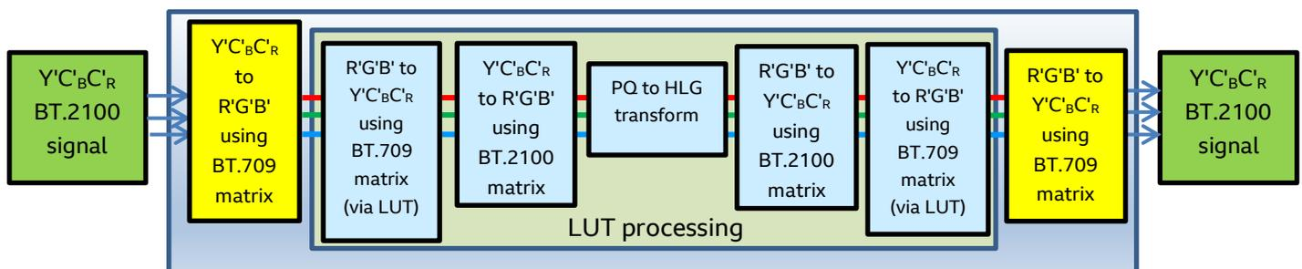
*Figure 7 - Example of colour-matrix compensation within a LUT.*
